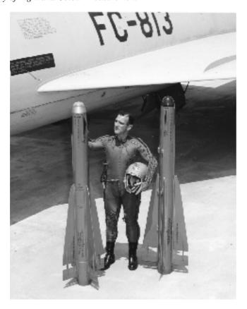
**Figure 9.1.** GAR-2A infrared Guided Aircraft Rocket (left) developed by US Air Force, beside James J O'Reilly, engineering test pilot for the Hughes Aircraft Company. In production from 1956, some 16 000 of the original design were produced. Reproduced with permission of HRL Laboratories, Malibu, CA.
