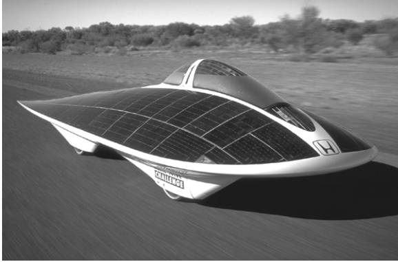
Honda's two seated Dream car is powered by photovoltaics. The Honda Dream was first to finish 3,010 km in four days in the 1996 World Solar Challenge. (Courtesy of Photovoltaics Special Research Centre, University of New South Wales, Sydney, Australia)
